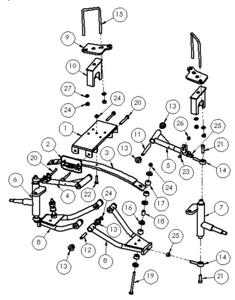
**16-010** Note: On this lift kit, the tie rod mounts on the spindles face to the front.
