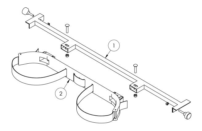
NOTE: EXTRA STRAP ALSO INCLUDED FOR WRAPPING AROUND THE BAGWELL BRACKETS TO SECURE LOWER BAGS
