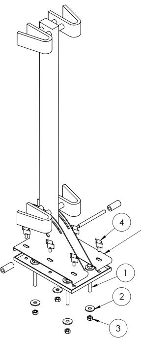
Gun Rack is packaged already assembled w/ Item#4, but these side plates for base will need to be removed to install the bottom plate to cart.
