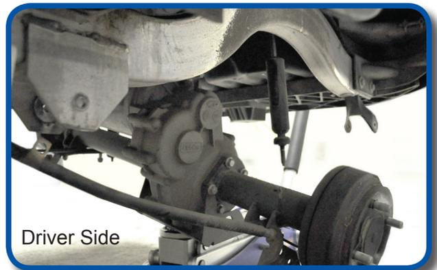
Use jack to lower axle and motor assembly. Reinstall leaf spring on top of axle using hardware retained from Steps 23 and 24.
