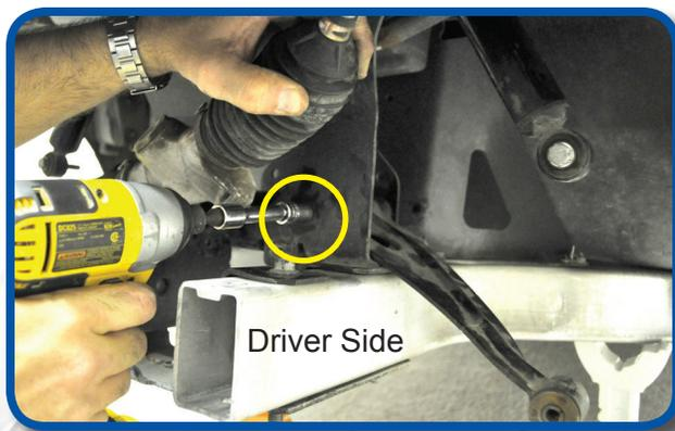
**Note: Grease all fitting before installing lift on Cart. 1 each on the upper A-Arms and 2 on each on lower A-Arms**
