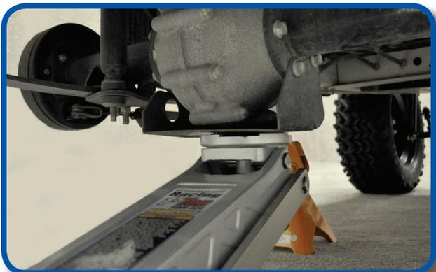
Using a 5/8" Socket remove the driver side U-Bolts. Once the U-Bolts are removed you can remove the lower bushing and shock using a 9/16" Socket. Retain shock hardware. Discard U-Bolts and nuts.
