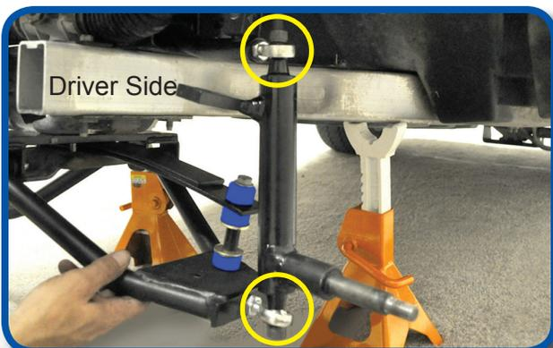
**Note: Before attaching spindles, adjust heim joints so there is approximately 1/4" of thread showing.**
