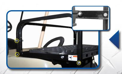
Attach upper armrests and seat back support bracket using hardware from Pack 3. Repeat process on the other side.
