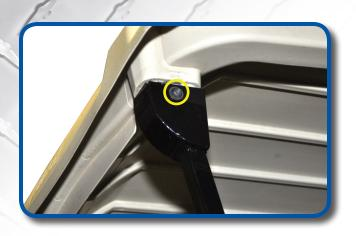
Using retained hardware from Step 2, attach rear struts to roof. Tighten all hardware.
