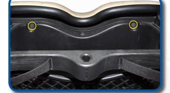
Remove upper rear canopy strut hardware. Use a prop to support canopy. Retain hardware.
