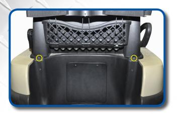
Remove hardware from base of basket. Two bolts are located in the rear and two bolts located in the front. Retain hardware.
