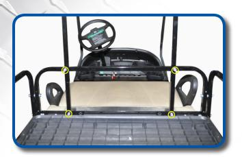
Attach rear struts to seat back support bracket using hardware from Pack 4.
